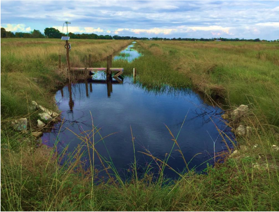
Photo 1: Instruments measure water inflows/outflows and phosphorus concentrations in water used for grass growth on Buck Island Ranch. Photo credit: Amartya Saha
